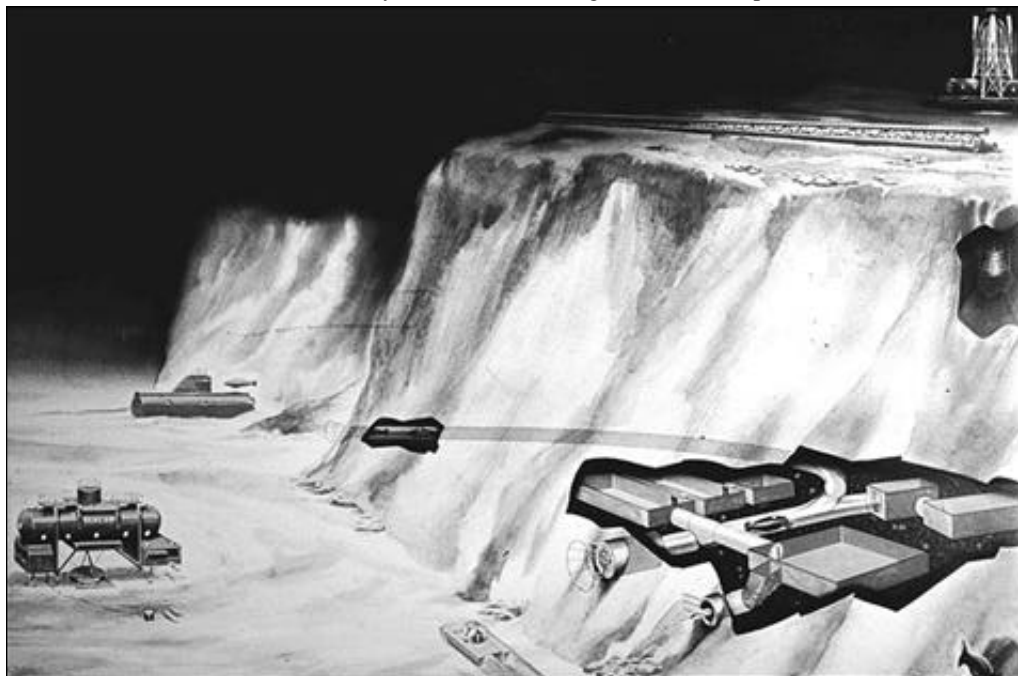
Illustration 2. Artist's depiction of Rock-Site Concept. Here you can see an undersea installation inside a sea mount, with locks for small submarines to come and go. A drilling derrick is on top of the mount, at upper right. The long tubular array on top of the mount could serve as a long-wave radio transmitter (ELF) or as a mechanism for water desalination and/or oxygen generation. (Source: US Navy)
